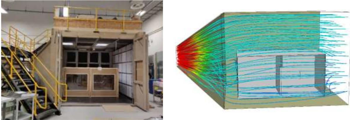
Figure 1. Gas leakage and accumulation test facility
