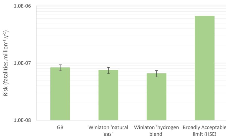
Figure 7. Individual risk associated with the conveyance of hydrogen blends
