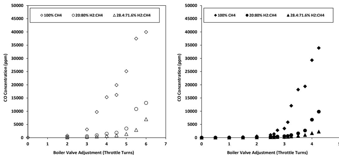
Figure 5. CO production during fault conditions (left – boiler A, right – boiler B)
