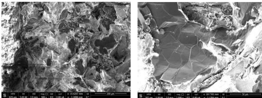
Figure 6. Fracture surface of cast iron specimen
