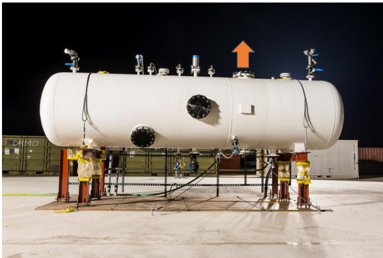
Figure 1. Photo of JR II ten ton release tank. The arrow depicts the upward jet release location at the top of the tank used in Trial 8. The bottom of the tank is 1 m above ground level.
