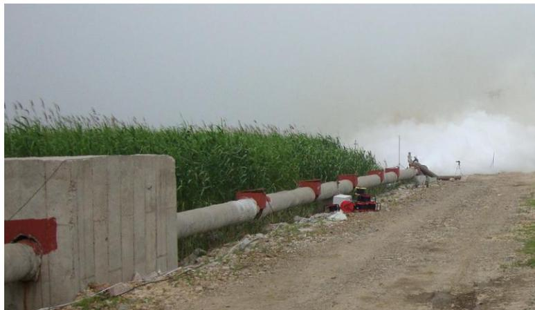
Photographs of the large-scale CO<sub>2</sub>PipeHaz pipeline test facility during pipeline rupture tests in China. At 250m long and 0.23 m i.d, it is the longest fully instrumented CO<sub>2</sub> test pipeline in the globe fed from 7 MW post combustion power plant.
